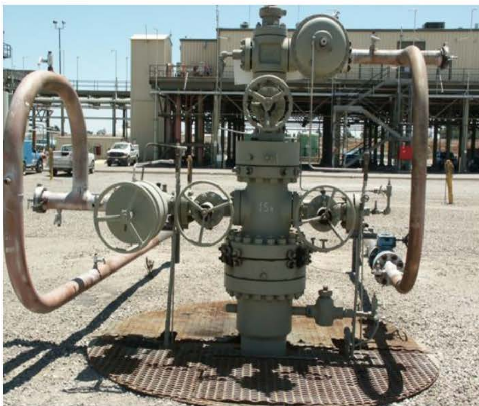
Figure J-1. A Typical PG&E Christmas Tree.
