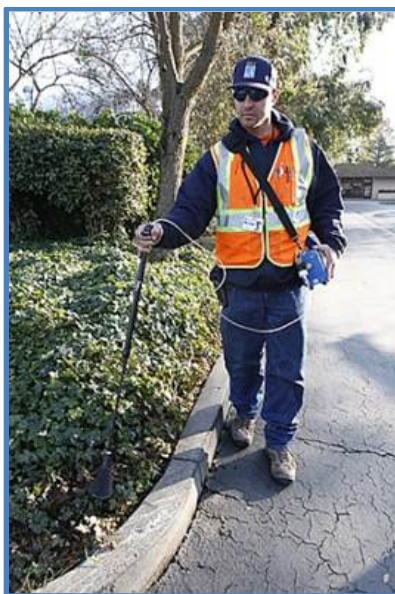
Figure 2.6 PG&E Leak Survey
