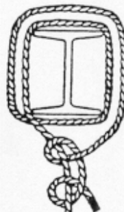
Bad Practice— Steel can cut rope
