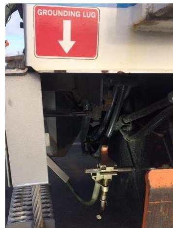
Figure 8.2 – Ground Clamp Attached
