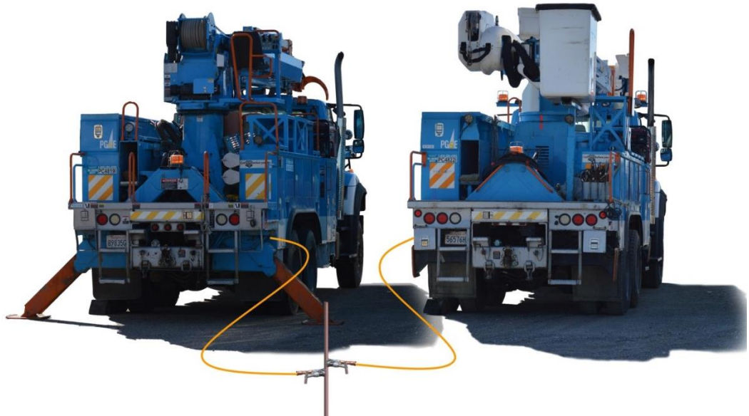
Figure 8.3 - Multiple Vehicles Connected to a Common Ground Source
