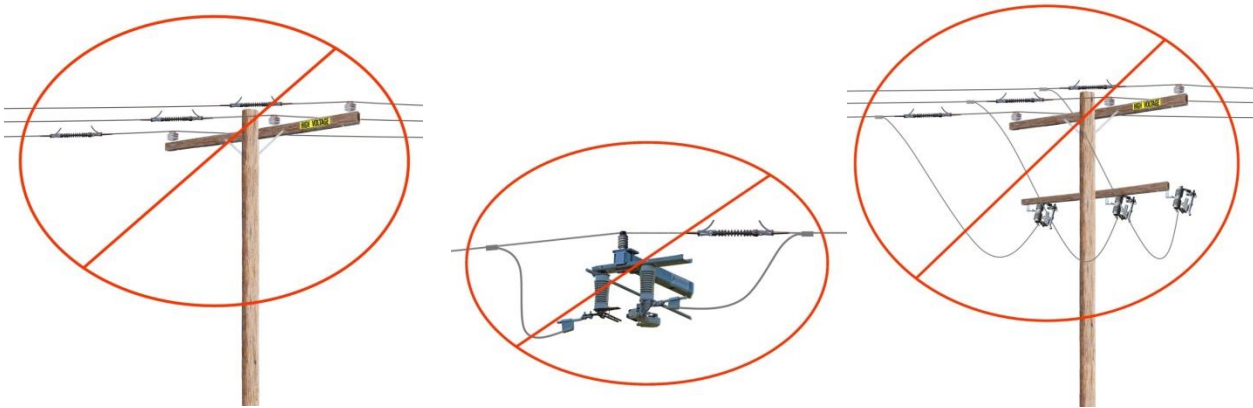
Figure 5.12. Sectionalizing Devices that Utilize a Single Strain Insulator
