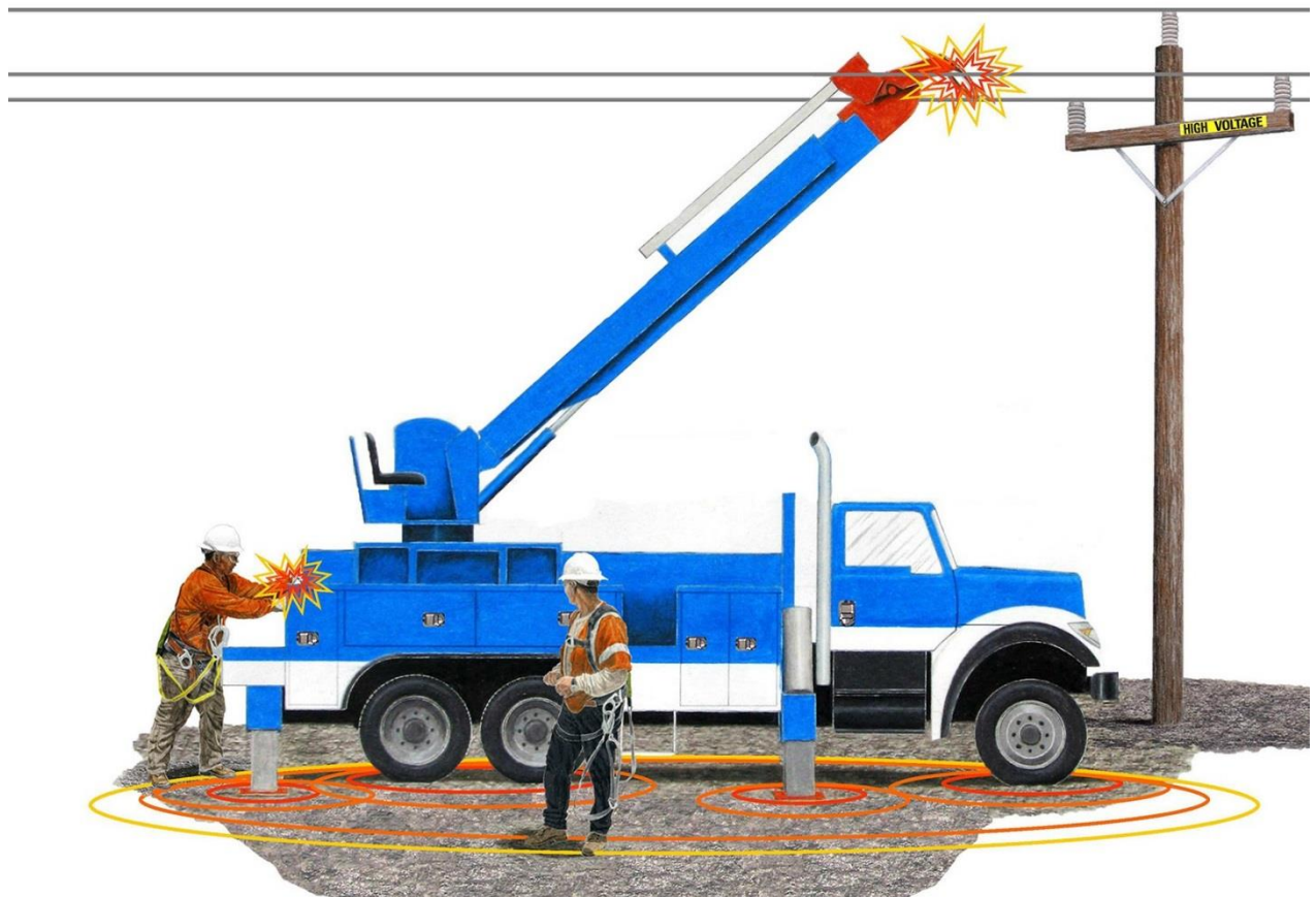
Figure 2.2. Step and Touch Potential
