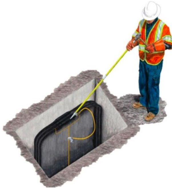
Figure 6.4. Cable Spike Model 1710: Tool Setup.
